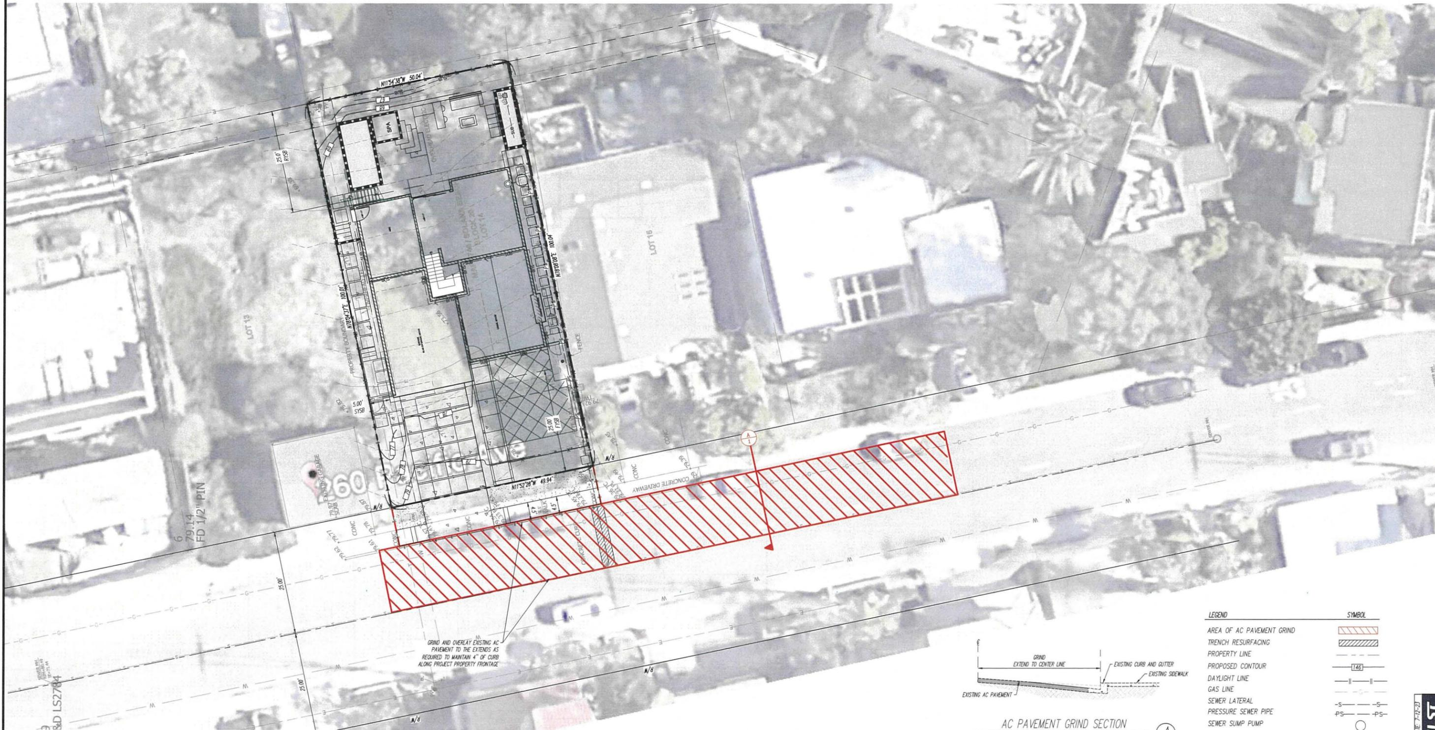
GRIND AND OVERLAY EXISTING AC PAVEMENT TO THE EXTENTS AS REQUIRED TO MAINTAIN 4" OF CURB ALONG PROJECT PROPERTY FRONTAGE
