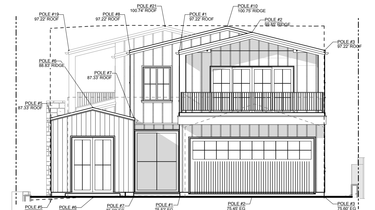
NORTH ELEVATION - STORY POLE SCALE: 1/8" = 1'-0"
