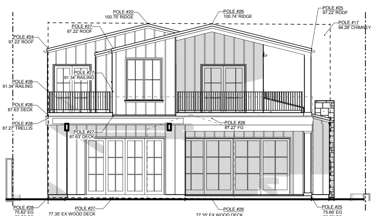
SOUTH ELEVATION - STORY POLE SCALE: 1/8" = 1'-0"
