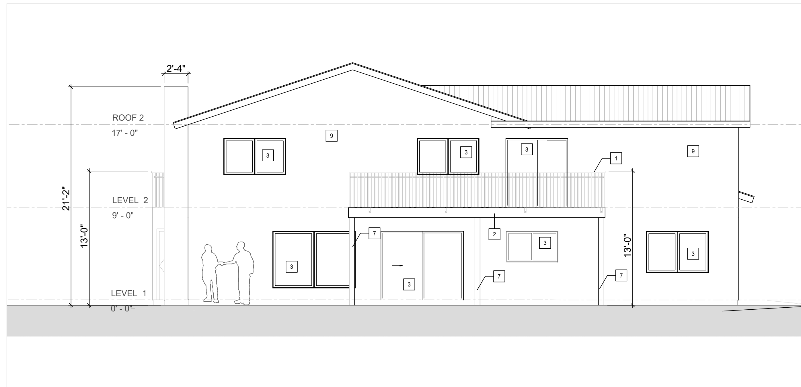
SOUTH REAR EXTERIOR ELEVATION EXISTING 3/16"=1'-0"
