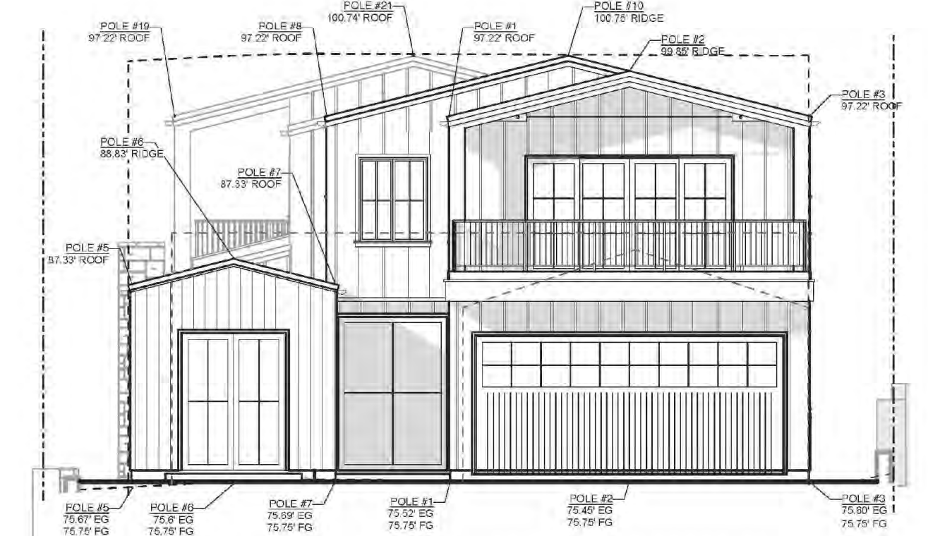
NORTH ELEVATION - STORY POLE SCALE: 1/8" = 1'-0"
