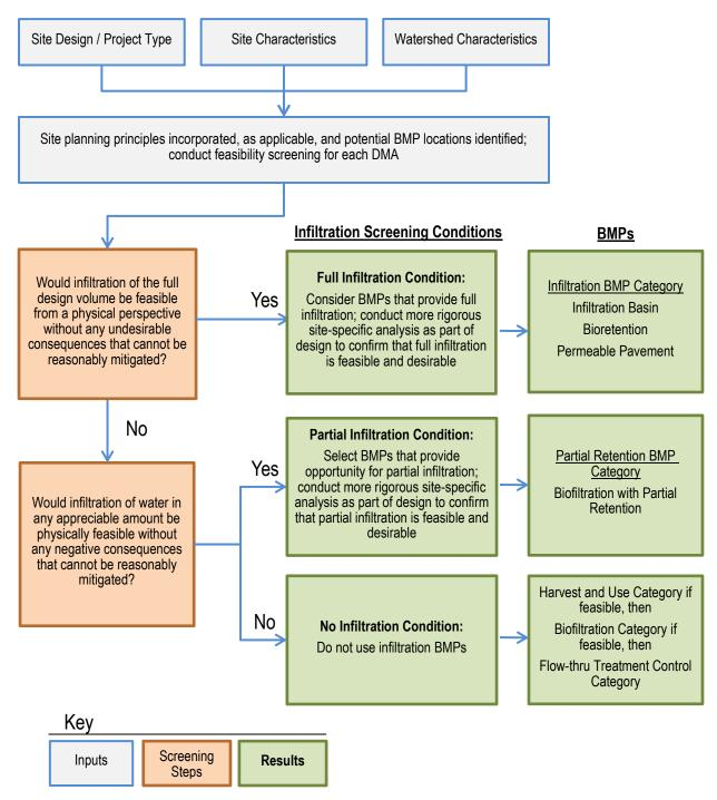
FIGURE 5-5. Infiltration Feasibility and Desirability Screening Flow Chart
