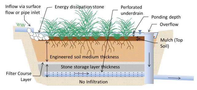
FIGURE 5-9. Schematic of a Typical Biofiltration Basin
