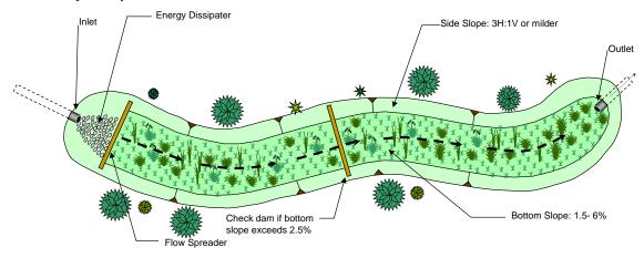
FIGURE 5-10. Schematic of a Vegetated Swale
