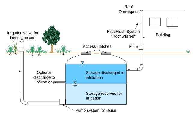
FIGURE 5-6. Schematic of a Typical Cistern
