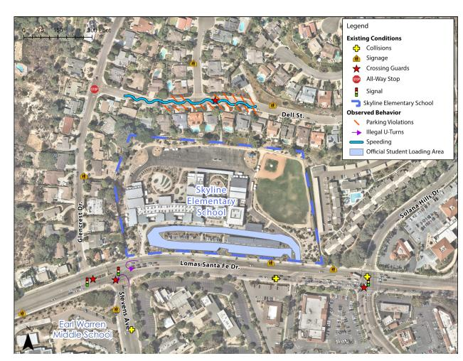
FIGURE 4.2.16. EXISTING ROADWAY NETWORK, OBSERVED VEHICLE BEHAVIOR, AND CONDITIONS.
