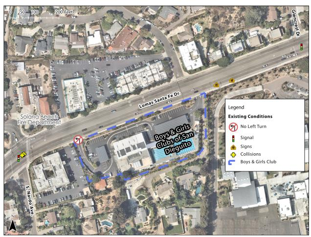
FIGURE 4.4.13. EXISTING ROADWAY NETWORK AND CONDITIONS.
