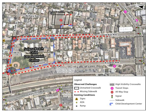
FIGURE 4.9.5. EXISTING PEDESTRIAN CONDITIONS AND OBSERVED CHALLENGES AND GAPS IN THE NETWORK.
