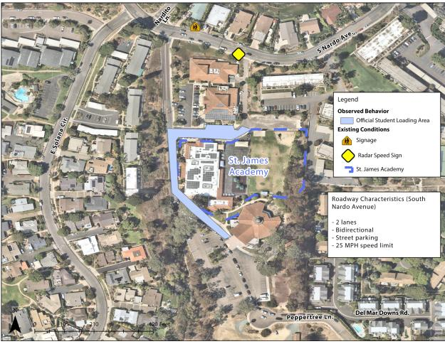
FIGURE 4.6.12. EXISTING ROADWAY NETWORK, OBSERVED VEHICLE BEHAVIOR, AND CONDITIONS.
