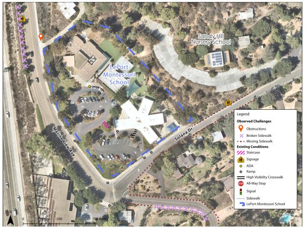
FIGURE 4.8.5. EXISTING PEDESTRIAN CONDITIONS AND OBSERVED CHALLENGES AND GAPS IN THE NETWORK.
