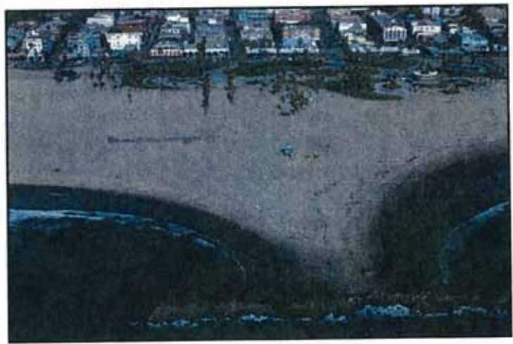
Figure 5.3. Offshore breakwater at Venice where beach has widened in protected area behind breakwater (2004). Photo © Kenneth and Gabrielle Adelman, California Coastal Records Project, www.Californiacoastline.org
