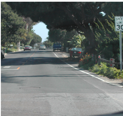
The above street has a painted edge stripe. Visually reducing the width of the road may help slow down some driver. This is an example of a non-physical improvement.
