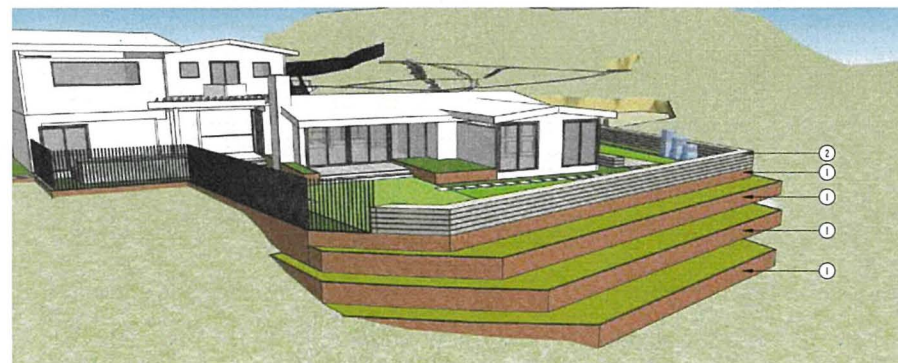
3. STACKED STONE WALL TYPES 1 AND 2
